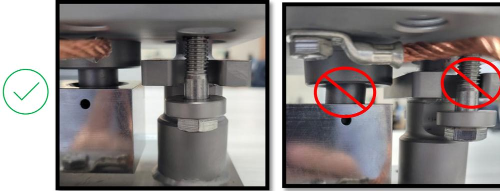
TOP PLATE VIEW: When aligned correctly, the pin is centered in the top plate.
