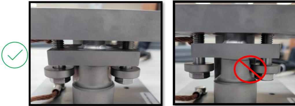
**SIDE VIEW:** When properly aligned, liftoff bolts will be centered in the machined center post cavity.
